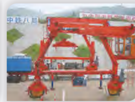
Railway Girder Machine
